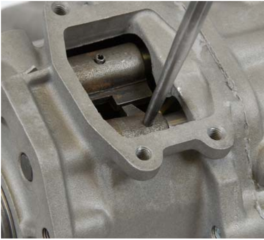
Step 12 Align the shift rail hole and the shift fork hole with each other using a long pin punch.
