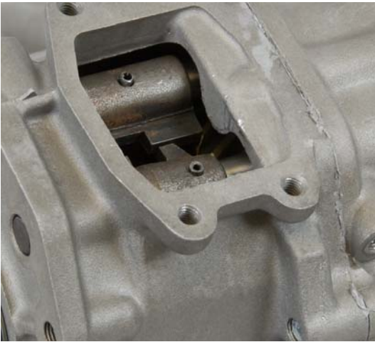
Step 14 Firmly tap in the roll pin until it is nearly flush.
