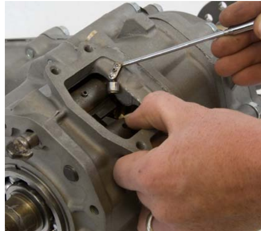
Step 5 Slide the drivers side shift rail forward until it stops. Insert a magnet under the shift rail to catch the roll pin.
