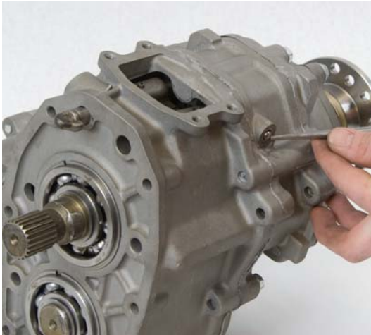
Step 4 Using a magnetized long pin punch remove the detent ball.
