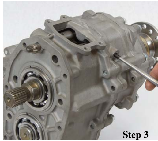
Step 3 Using a magnetized long pin punch, remove the detent spring. If a magnetized pin punch is not available, roll the t-case over for the spring to slide out of the hole.
