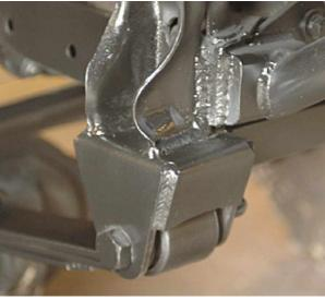
10) Install leaf springs with military wrap (full double wrapped) end forward into the front hanger. Use shackle kit provided with kit to attach the rear end of the springs to the frame. Apply a small dab of axle grease to the threads of the shackle bolts before installing locknut. Grease shackles with standard grease gun. Shackles can be installed with grease fittings facing inside or out.
