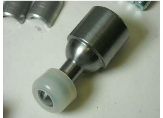
13. Install the transmission shifter into the shifter tower making sure to line up the shifter extension into the shift mechanism in the transmission.
