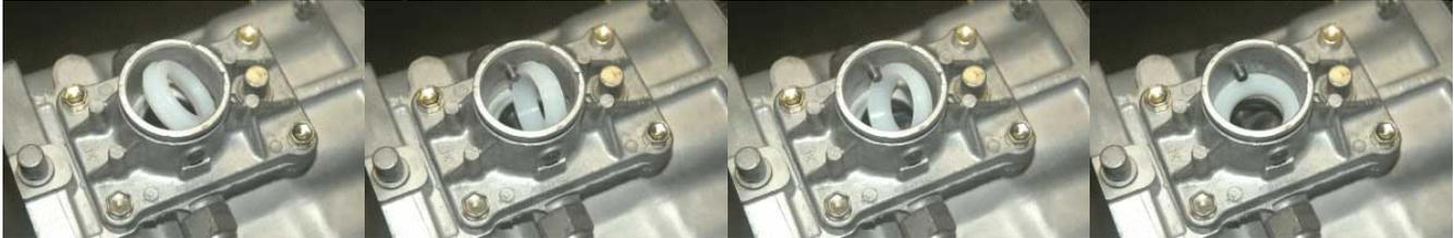
**12.** Install the shifter extension onto the transmission shifter. It will also use the two keepers to position and retain the extension onto the shifter.
