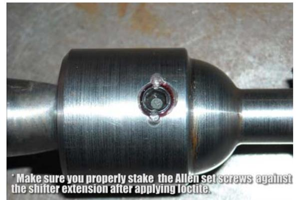
**ATTENTION:** After installing the short shifter there should be no excessive play or travel in the shifter. If, after time, you notice more play in the shifter, remove the shift tower and inspect the shift extensions to verify that the set screws have not come loose. If the set screws come loose they can fall into the transmission and cause transmission failure.
