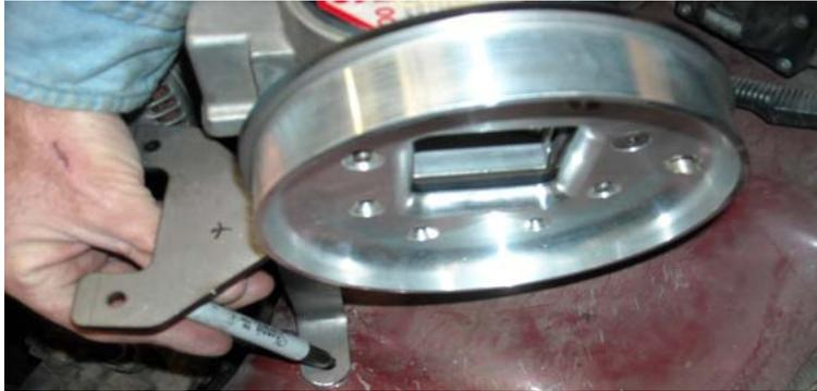
13. Remove the bracket assembly and center punch the second mounting hole that you just marked.
