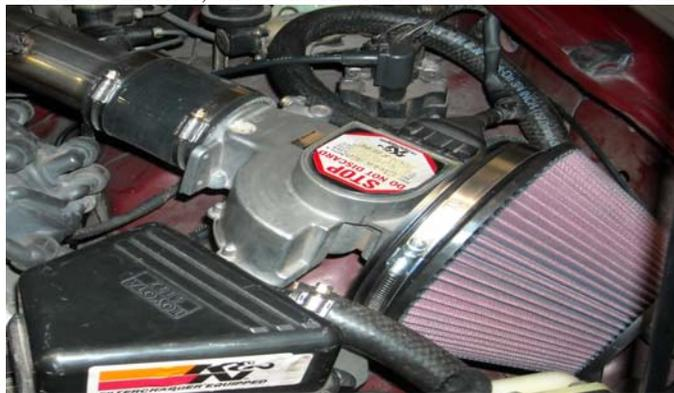
22. Adjust as needed and tighten hose clamps.
