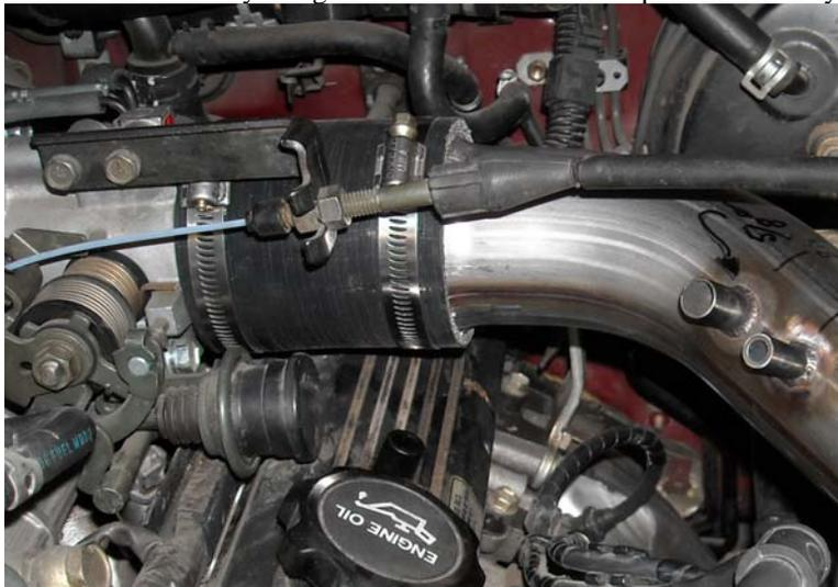
10. Install the mass airflow sensor (already installed onto the bracket assembly from step 7) to the intake tube using the other silicone coupler, do not install clamps on this side yet.
