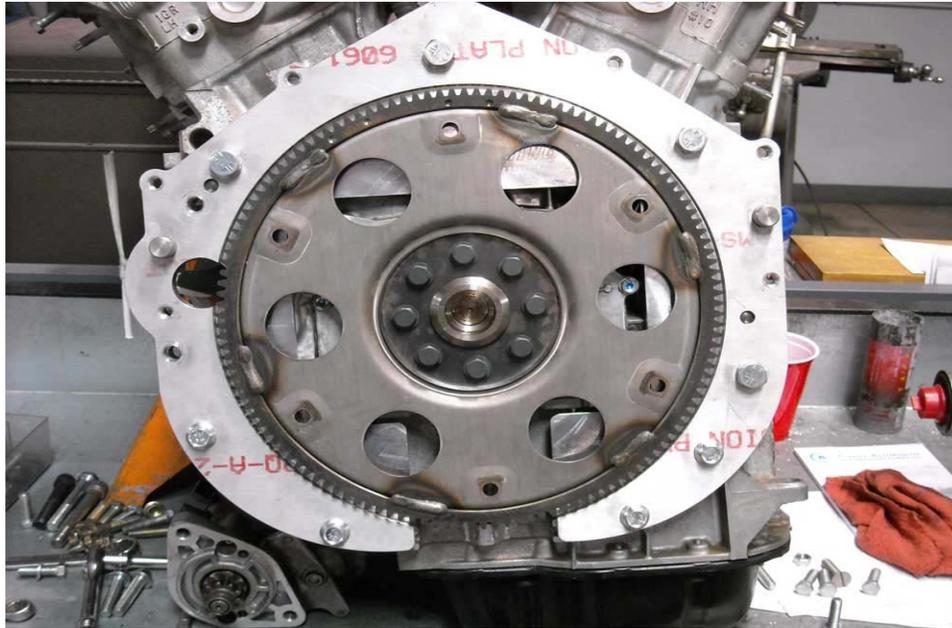
6. We have provided a torque converter pilot collar to support the nose of the torque converter and to keep it centered with the crankshaft. If you are custom making a torque converter then we would recommend having the torque converter made with a longer nosepiece to align itself in the crank, which will eliminate the need for this pilot collar. If you are not using a custom-made torque converter then follow step 7 for installation of the pilot collar.
