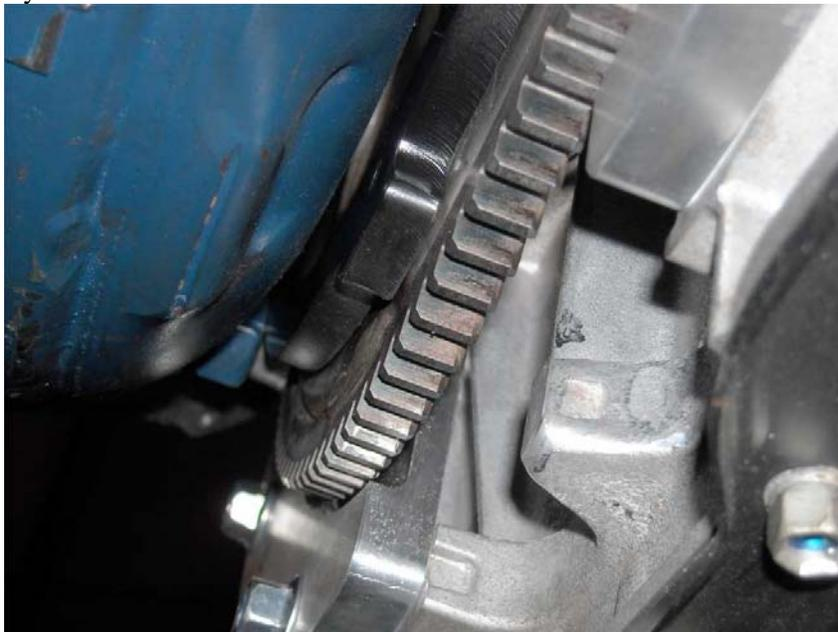
12. Install the starter using the M10x1.25 x 45mm flange bolts provided. This is where you will use the access hole you drilled in the bellhousing earlier. Tighten bolts.
