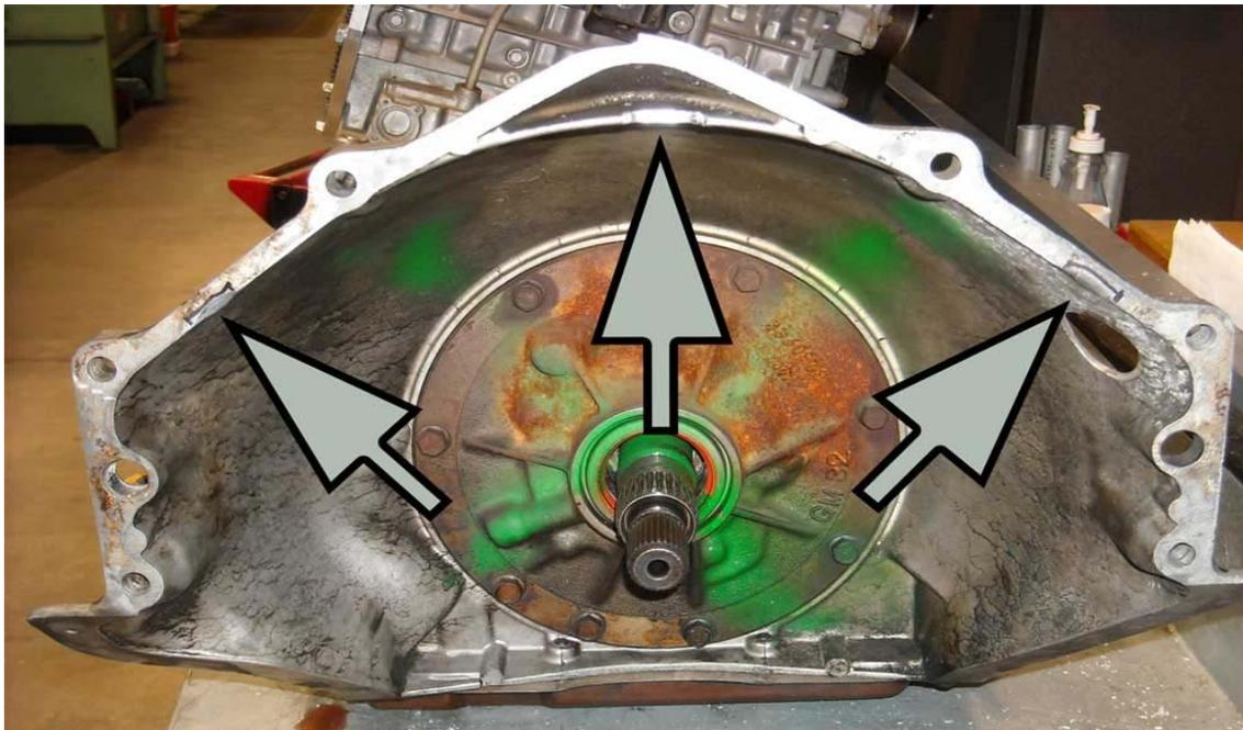
2. Using a hole saw, drill a 1- 1/2" hole in the bellhousing as shown for access to the top starter bolt. Grind or file as necessary for proper access for a 14mm deep socket. Use the starter as a template for proper hole location. **Failure to follow this step will result in needing to remove the transmission to access the top starter bolt! If you plan on removing the starter without removing the transmission, this step is crucial!**
