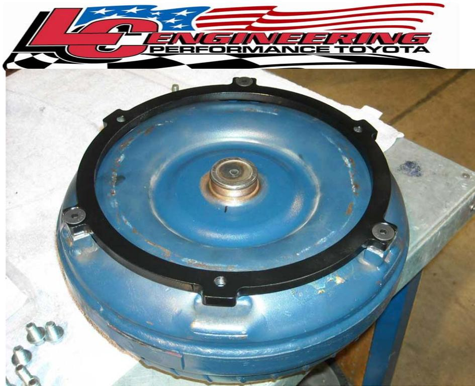
9. Install the converter into your prepared transmission. Lube the front seal and make sure the converter registers completely on the input shaft. **Do not force the converter onto the shaft! Make sure the converter is fully seated on the shaft! Failure to properly install the converter will result in front pump damage!**
