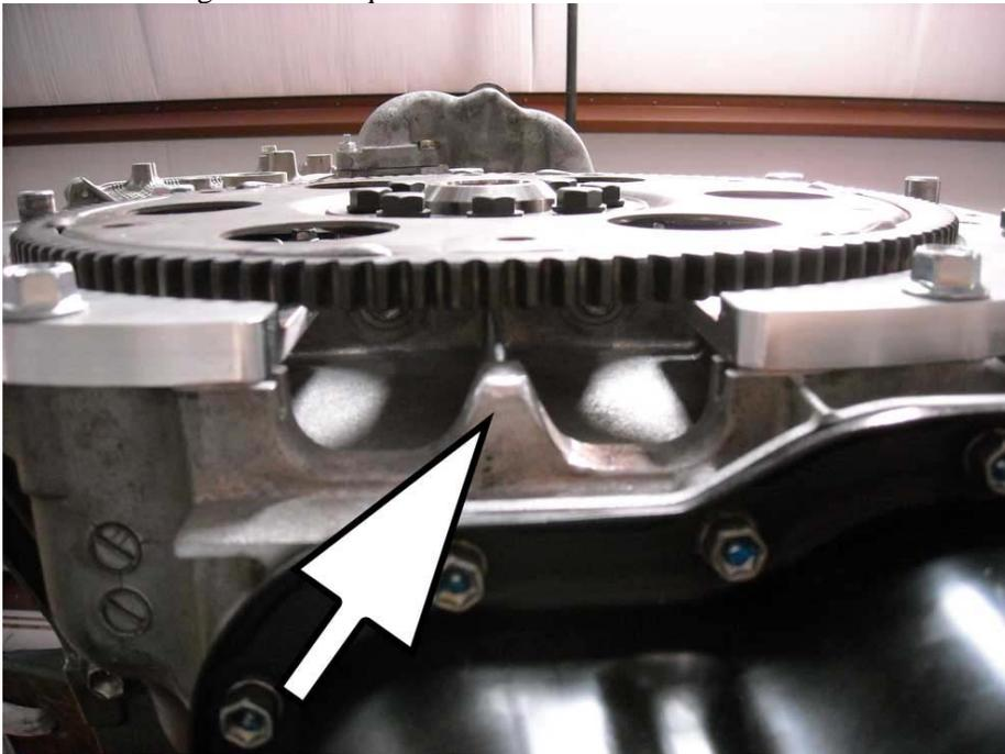
4. Install the adapter plate to the engine block using the hardware provided. 4 M12x1.25 x 30mm bolts with flat washers and 4 M10x1.25 x 30mm flange head bolts. Use thread locking compound on the threads and tighten.
