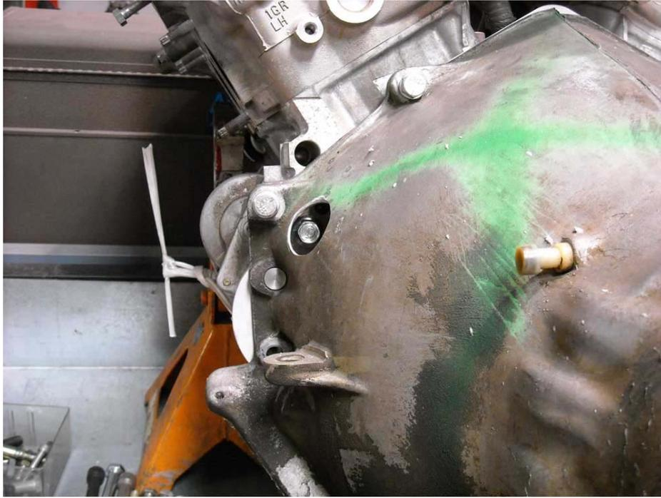
3. Clearance the bottom of the engine block as shown for torque converter bolt access. The more clearance, the easier it will be to install and tighten the torque converter bolts.
