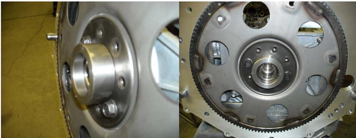
8. Install the torque converter adapter ring to the converter using the 3 allen-head bolts provided. Use thread locking compound on the threads and tighten. Use the 3 outer diameter holes for the converter.
